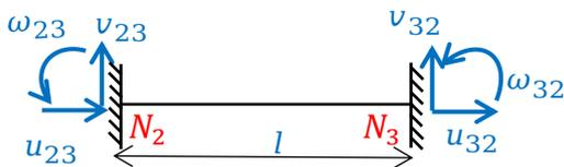
$$\left\{ \begin{array}{l} N_{23}^* = \frac{EA}{l} u_{23} - \frac{EA}{l} u_{32} \\ V_{23}^* = 12 \frac{EI}{l^3} v_{23} + 6 \frac{EI}{l^2} \omega_{23} - 12 \frac{EI}{l^3} v_{32} + 6 \frac{EI}{l^2} \omega_{32} \\ M_{23}^* = -6 \frac{EI}{l^2} v_{23} + 4 \frac{EI}{l} \omega_{23} + 6 \frac{EI}{l^2} v_{32} + 2 \frac{EI}{l} \omega_{32} \end{array} \right. \Rightarrow \left\{ \begin{array}{l} N_{23}^* = 2 \frac{EA}{l} U_2 \\ V_{23}^* = 0 \\ M_{23}^* = 2 \frac{EI}{l} \Omega_2 \end{array} \right.$$
