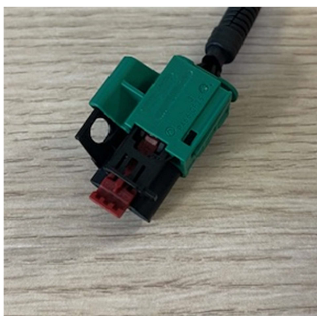
E-Plug de désactivation Position 2
