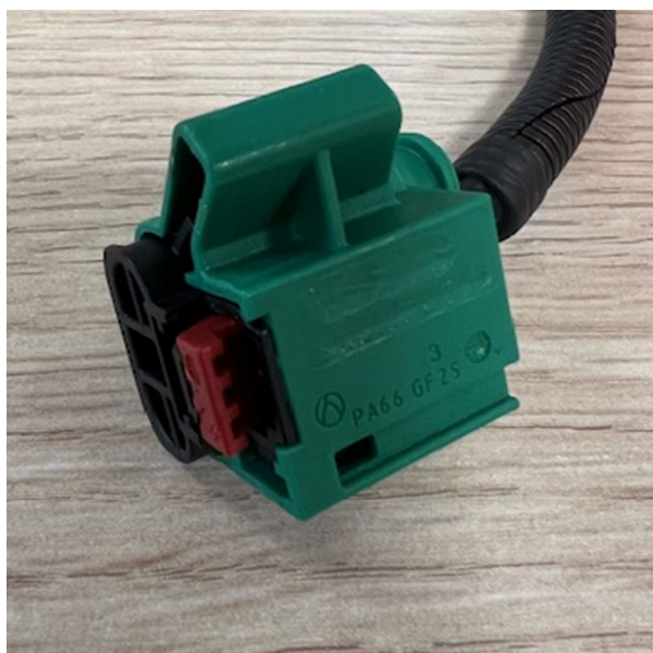
E-Plug de désactivation Position 1
