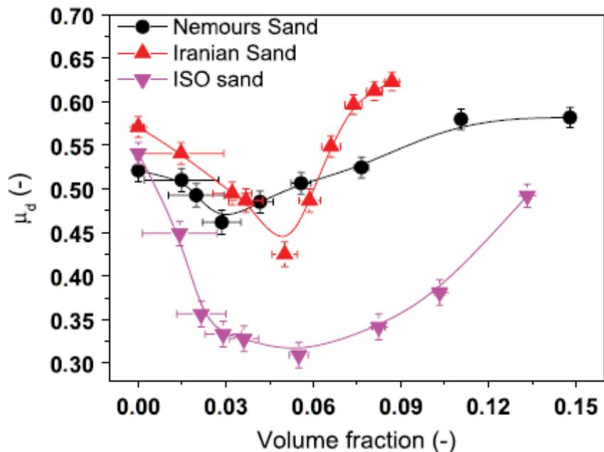
**Figure 6 : Friction coefficient for different types of sand**
