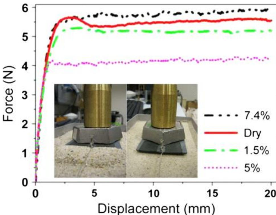
Inset: Picture of the setup. The picture on the left was taken while sliding over dry normalized sand. The picture on the right was taken while sliding over normalized sand wetted with 5% water (volume fraction). In the dry sand, a heap clearly builds up in front of the sled. The 11×7.5cm sled is made out of PVC with rounded edges (as the Egyptian sled) and a roughness of 35µm with sandpaper on its bottom;
