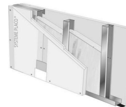
**CLOISON PLACOSTIL® SAA 160 - 2XPLACOPLATRE® BA 13 - EI 60 - 62DB - 3,40M**
